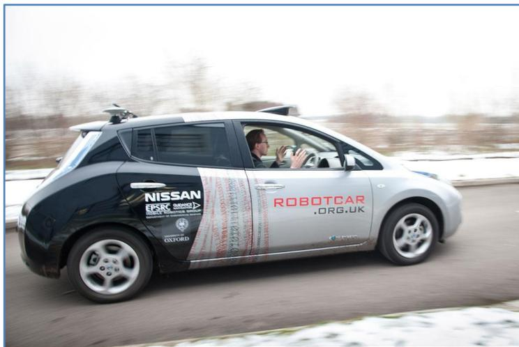
and Physical Science Research Council has helped the University of Oxford with the [Robotcar](#) project. Collaborating with Nissan and MIRA, the focus of the research is on an infrastructure-free solution to vehicle autonomy. Using on-board sensors and a training / learning routine, the car interprets a fusion of data from the sensors to recognise its surroundings and navigate accordingly. Pedestrians, cyclists
